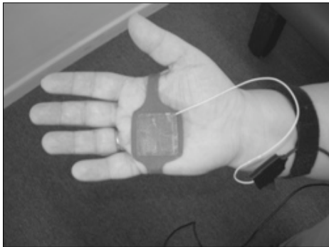
The pressure pad installed prior to trial.
