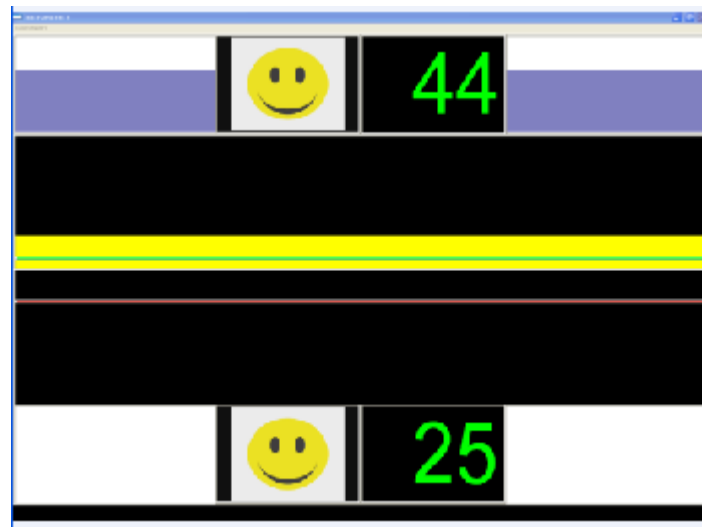
Figure 4: Feedback screen. The blue area indicates the participant should modulate the signal in upward direction. The yellow bar signal reflects the integrated EEG or GSR signal. The numbers show the percentages correct for upward direction (44%) and downward direction (25%). The smileys pop up when the participant exceeds the threshold bar (horizontal lines in middle of the screen) in the indicated area. When the signal exceeds threshold for more than two seconds, the participant hears a reinforcing sound.
