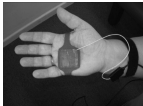
Illustration 3. The pressure pad installed prior to trial.
