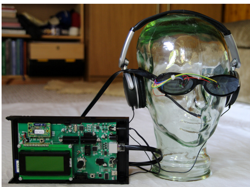
Figure 5. The complete stimulation unit consists of the MediTrain device (version 2) plus headphones and 3 colour LED glasses. This device can receive data from the PC (Thought Translation Device Software) or directly from a portable EEG amplifier such as the PET device as shown on the right.
